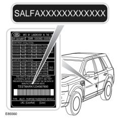
The Vehicle Identification Number (VIN) is shown on a label attached to the driver's door pillar. The VIN on the label should match the VIN recorded in the Passport to Service, and the VIN visible through the front windshield.
